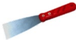
Paint scraper YORK® type 870 high carbon hardened steel, flexible ground blade, plastic handle (PP), riveted 12 sizes 30 - 160mm
